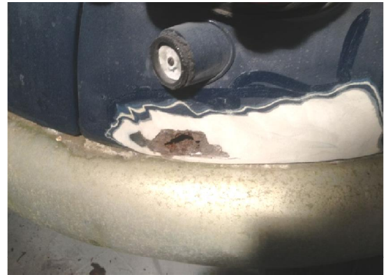
Some of the problems that emerged when the sander was put to the bodywork
