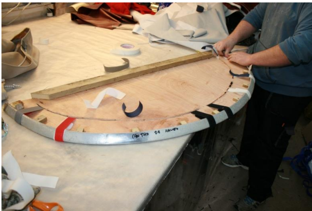
Polishing 50 year old partly pitted aluminium is a frustrating and thankless task with a result that will effectively continue to corrode and get thinner as time goes by--despite painting/ sealing the reverse sides
